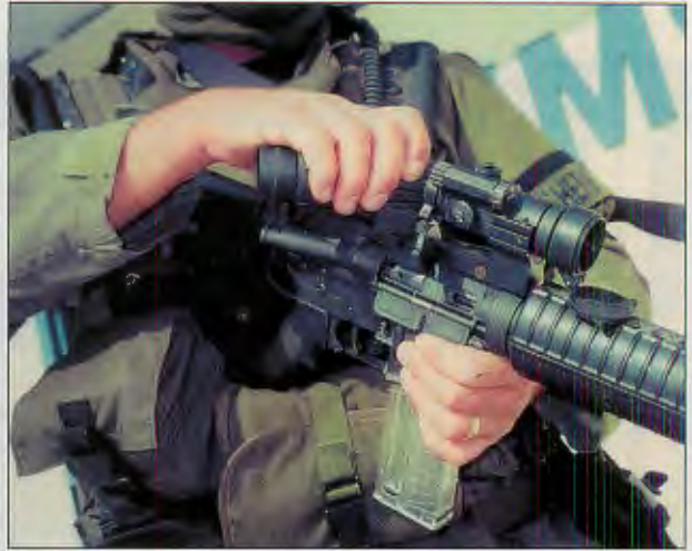
This SWAT officer demonstrates how easy it is to remove the Aimpoint 3X Extender from its mount, leaving the Comp M3 in place.
