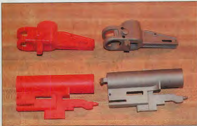
Wax injections of the AA-12's sight tower and bolt result in perfect steel counterparts during the precision investment-casting process.
